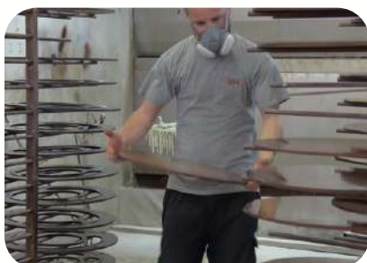
Drying after spray painting
