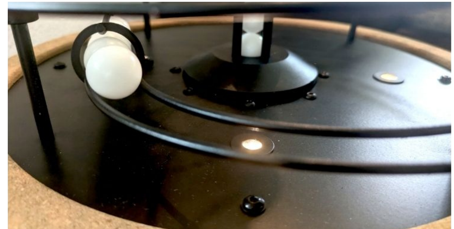
BIG M tracks are illuminated by three LED spotlights in the base
